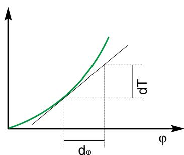
Dynamic torsional rigidity  $C_{T\text{din}}$  is the first derivate of the nominal torque of half coupling in respect to the torsion angle.  $\varphi$  is the torsion angle of half coupling in respect to the second half. As a general rule,  $C_{T\text{din}}$  is greater than  $C_T$  and depends on the stress acting on the coupling.
