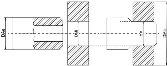
Interference fit shaft-hub connections can be achieved by cooling the shaft or heating the hub. This type of connection is not widely used for the following reasons:
